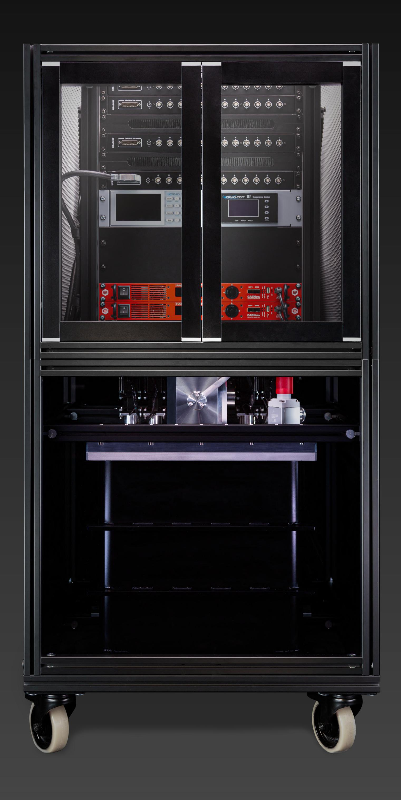
The S-Type Essential is a versatile, rack-mountable sub-Kelvin platform designed for the operation of low-temperature electronic devices, such as single-photon detectors or light sources, or the integration of complex customer setups. In its standard configuration, the system provides continuous cooling at 300 mK and "one-shot" operation down to 100 mK – independent of the supply with cryogens.
