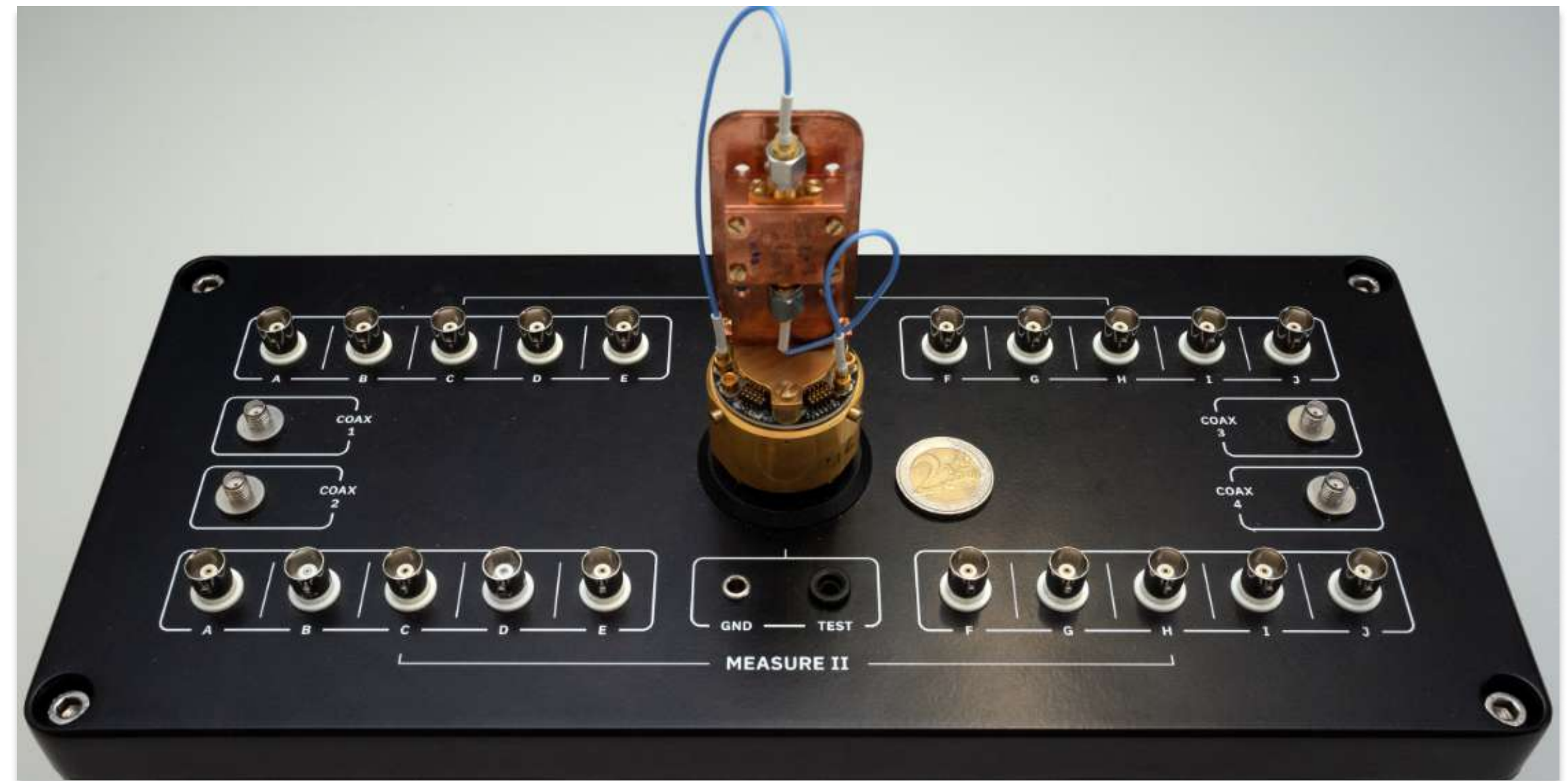
Picture of the OFHC copper box containing the resonator, mounted on the kiutra Sample Puck. The box is connected to the SMPM connectors on the Puck using flexible SMA to SMPM copper lines. The Puck is placed on a kiutra Sample Puck Station for preparation and room temperature testing.
