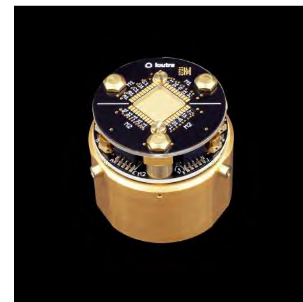
Sample Carrier Pad 40 mounted on RF Puck 36
