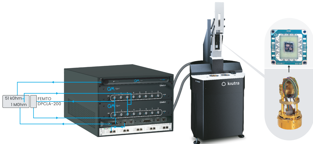
Figure 1: Measurement setup showing the room temperature electronics connected to a kiutra LTR and an optical microscope image of the CBT sample. The dimensions of the chip carrier (daughterboard) sample mounting area are 14 mm x 11 mm. The CBTs, bond-wired to the daughterboard, are mounted on the Qboard-II and connected to the kiutra Puck 55, to load it into the cryostat.
